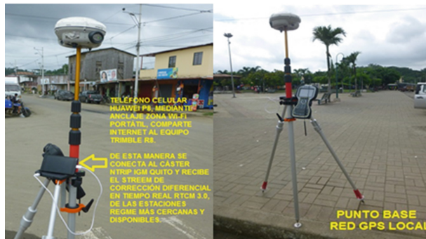
Fig. 6. Trimble R8 GNSS L1/L2 rover equipment (GPS + GLONASS) configured to connect to the Principal Caster using a cell phone as hotspot
